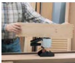
Gluing with the upper roller.
