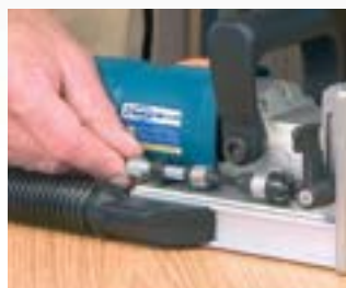
Quick adjustment of different slotting depths.
