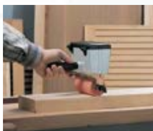
Gluing with vinyl (white) glues
