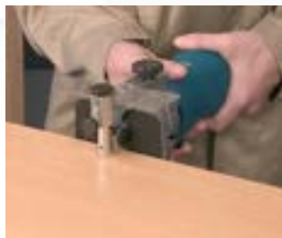
Excellent finishing when trimming laminates.
