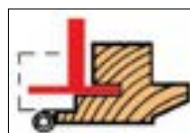
Slotting a window, hinges side.
