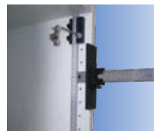
Drilling for placing invisible hinges.
