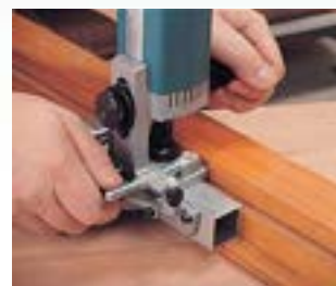
Slotting a window, lock side.
