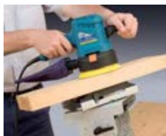
Folding and rotary adjustable support.
