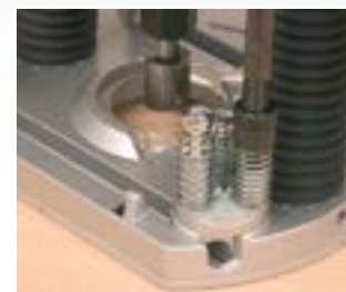
Quick adjustment of routing depth with 3 positions.
