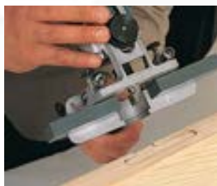
Placing hinges with the ZB93 head.
