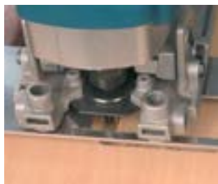
Guide ring for copying with template as a small router.
