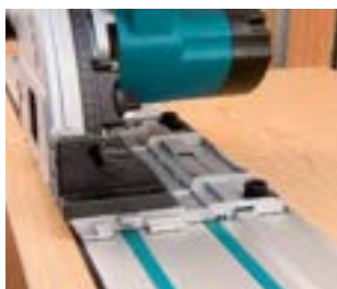
Precise gliding adjustment without lateral movement.
