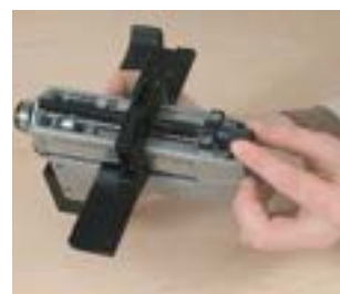
Micrometric regulation of the cutting width.
