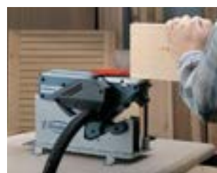
Planer stand. To be fixed to a workbench for using the planer in a stationary position.
