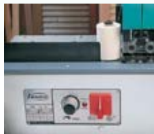
Electronic temperature regulation.
