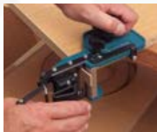
Cutting on both sides on straight panels.
