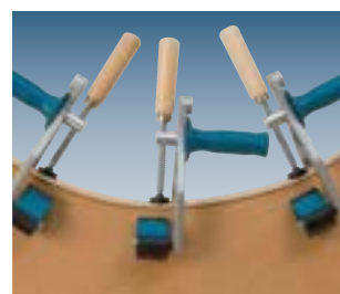
Fixing tapes on concave panels
