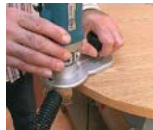
The CA56U trimming head enables uninterrupted trimming of the four edges of a panel. It has a large support base and an auxiliary holding knob, designed to give it perfect stability.
