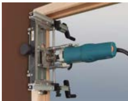
Making the upper recess on the frame.
