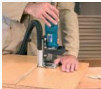
Joints in middle of board.
