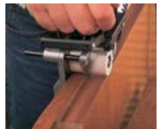
Banding the upper side of the lap.
