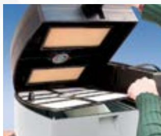
Double filter for microparticles. Automatic shaker for filter.
