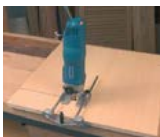
Trimming parallel slots.
