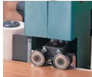
Power trimming unit: trimming both sides simultaneously.
