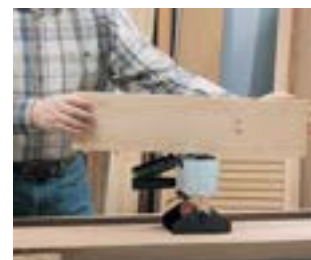
Gluing with the upper roller.
