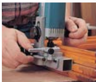
Slotting a window, flashing side.
