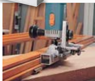
Slotting a window, hinges side.
